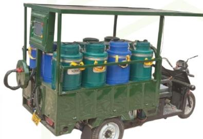
The Nomad EV/D is a rugged three-wheeler designed to deliver cold chain mobility and dispensing functionality in a single unit.
